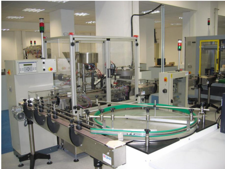
Automatic filling, line-ERM Training Centre, Faculty of Mechanical Engineering STU
